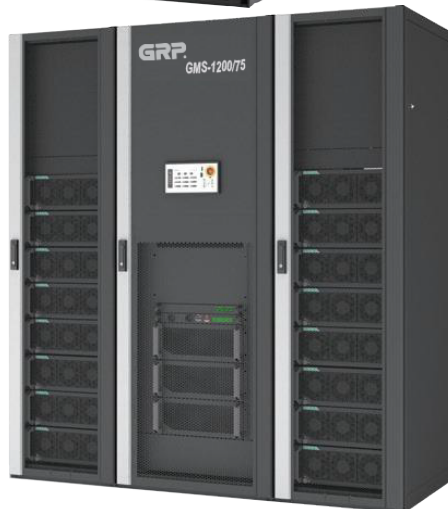
Model: GMS-1200/75 Max. Capacity of system: 1200KVA, Configuration: 16 slots Power module model: GM75, Power module capacity: 75KVA Dimension: 2000*1000*2200(W*D*H)mm, Standard cabinet: 19"
