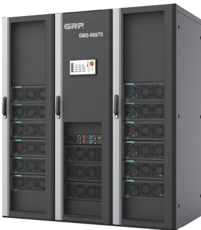
Model: GMS-900/75 Max. Capacity of system: 900KVA, Configuration: 12 slots Power module model: GM75, Power module capacity: 75KVA Dimension: 1800*1000*2000(W*D*H)mm, Standard cabinet: 19"
