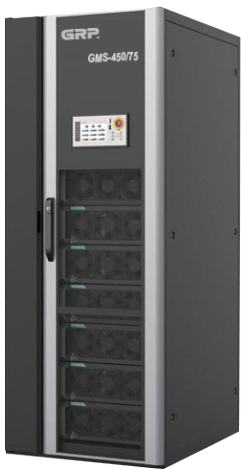
Model: GMS-450/75 Max. Capacity of system: 450KVA Configuration: 6 slots Power module model: GM75 Power module capacity: 75KVA Dimension: 900*1000*2000(W*D*H)mm Standard cabinet: 19"
